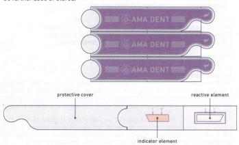
The reactive element is white color and the indicator element is light-orange. One or two samples from one patient can be tested at the same time.
