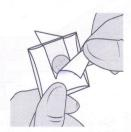
Place the AMA DENT segment into the slot of the heater for an exposure time of 10 minutes.
